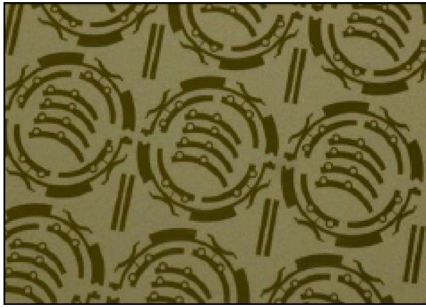
Fig. 5 Photo of X-ray mask for manufacturing of the mesoscale tilting pad gas bearings. Dark area is X-ray transparent material (represents the areas for bearing structures) and bright area is with X-ray absorber (Au film).
