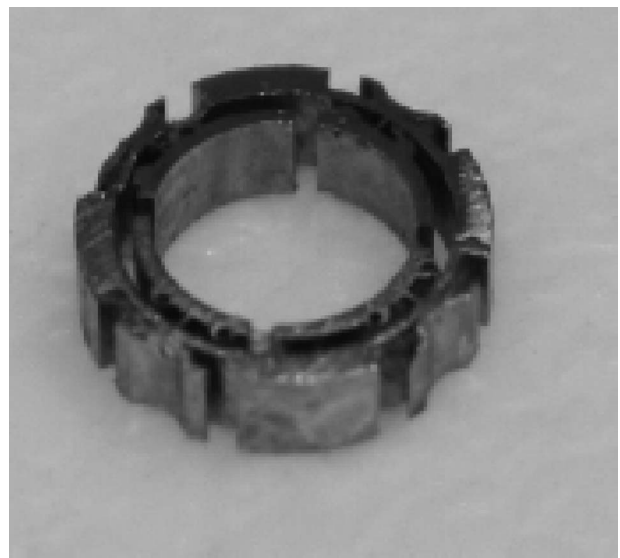
Fig. 7 Optical image of 2.0 mm thick mesoscale tilting pads gas bearing (a) 600,000 rpm, (b) 800,000 rpm, and (c) 1,000,000 rpm
