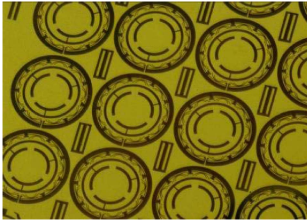
Fig. 6 Photo of an X-ray mask for manufacturing of the mesoscale foil gas bearings. The dark area is the X-ray transparent material (represents the areas for bearing structures) and the bright area is with the X-ray absorber (Au film)
